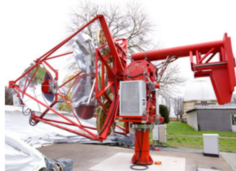
telescope prototypes, the Gamma-ray Cherenkov Telescope (GCT).
