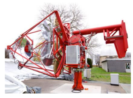
telescope prototypes, the Gamma-ray Cherenkov Telescope (GCT).
