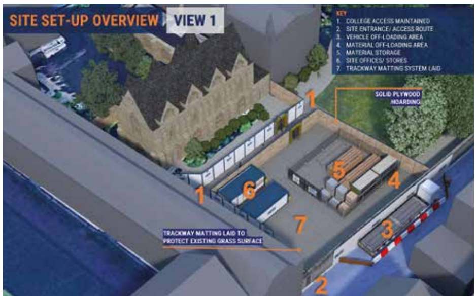
Image: Proposed plan showing access to building site, contractors' compound and protective hoarding
