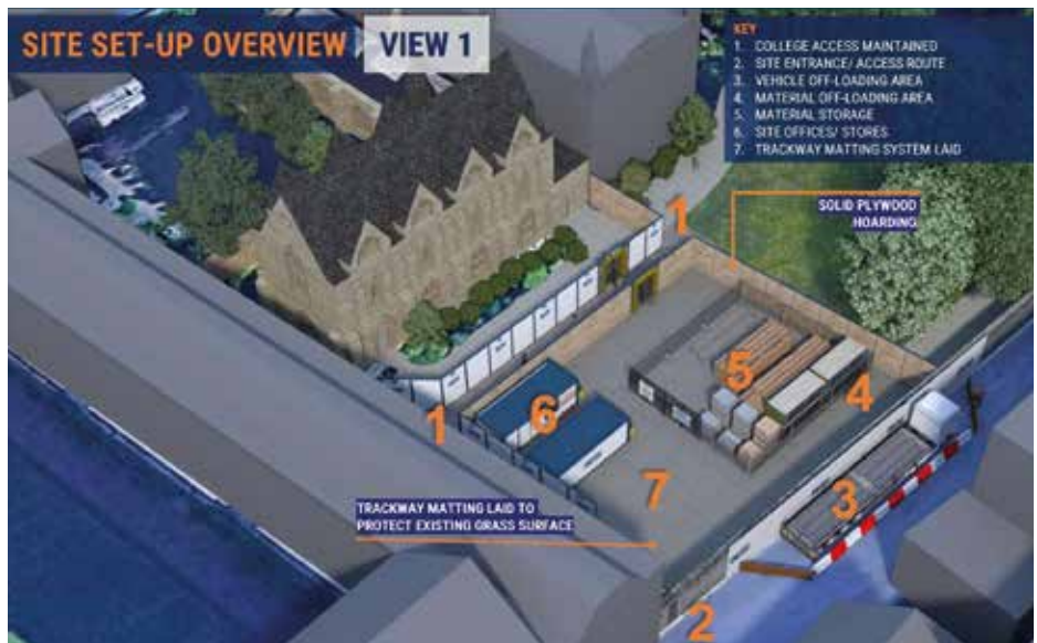
Image: Proposed plan showing access to building site, contractors' compound and protective hoarding
